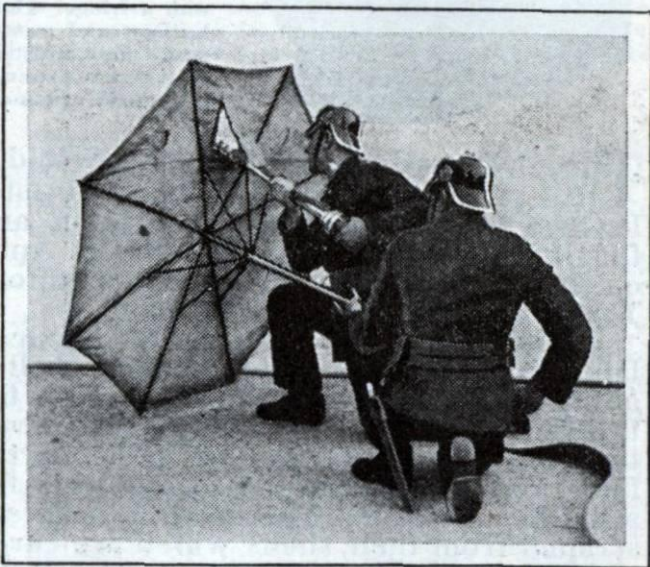
This large type of asbestos umbrella permits several hose nozzles to be thrust through it, protecting firemen from heat.
